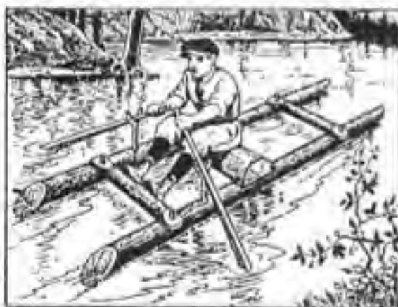
A Useful Boat, Built of Logs as a Catamaran Raft. Takes the Place of a Regulation Rowboat When the Latter is Not Easily Obtained
